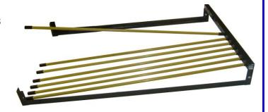
5. Take second 4' rod frame section (with plastic insert in place) and begin inserting each rod, one by one, into the support. Will be easier by keeping rod frame section at an angle.
